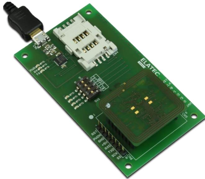
The Mini Reader is a device for reading and writing RFID transponders. It can communicate with a large range of transponder types in the frequency range of 13.56MHz.
